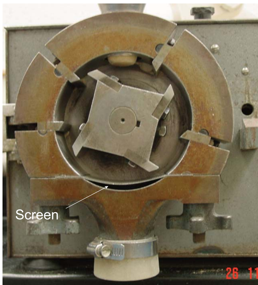
Photo G1: Standard Thomas-Wiley Mill, with chamber dimensions of 20 cm diameter and 7.6 cm depth.
